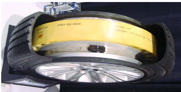
Figure 2. Michelin PAX run-flat design.
